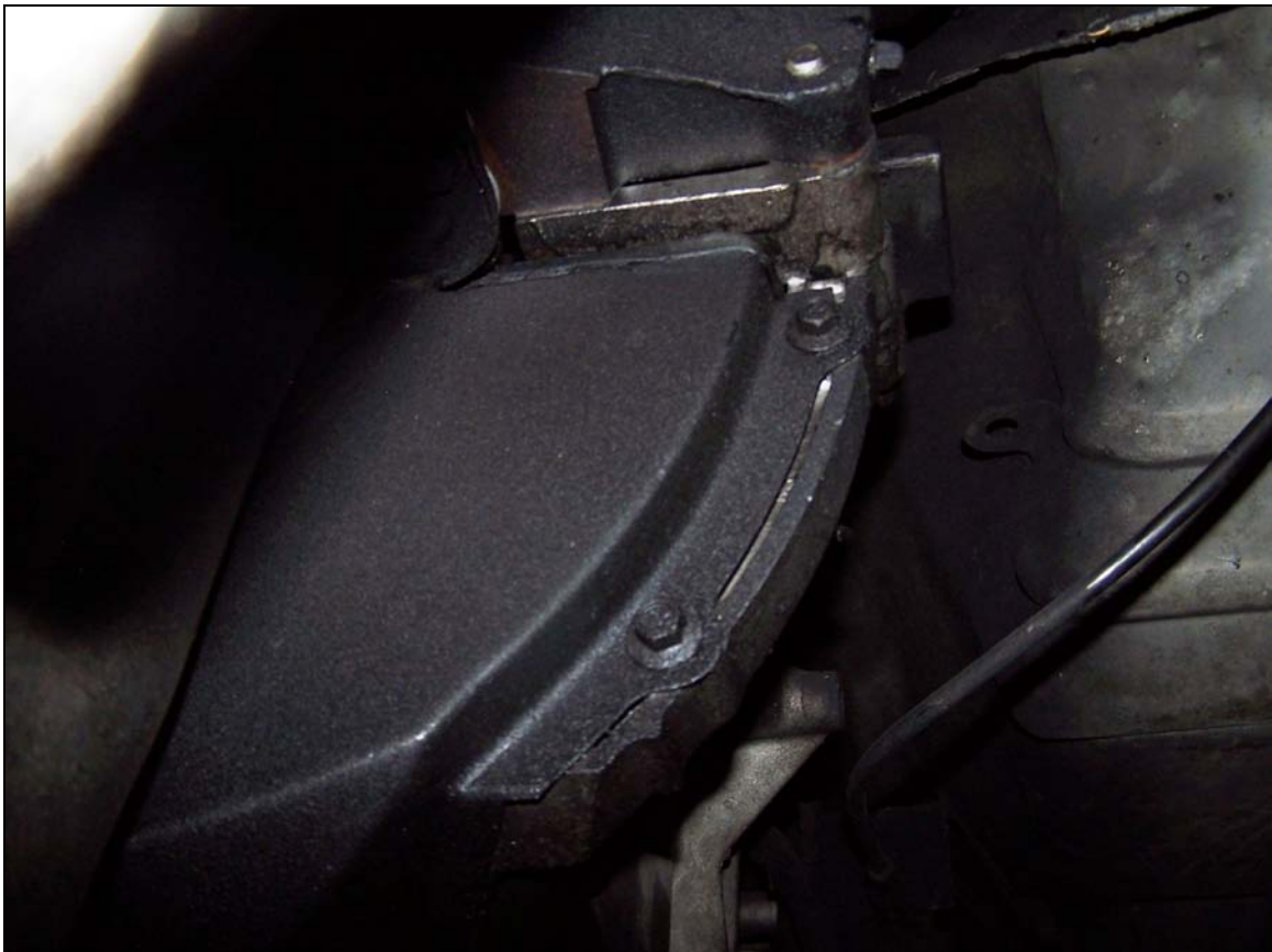
Image 1 – Automatic Trans Inspection Plate – Driver Side Bolts
