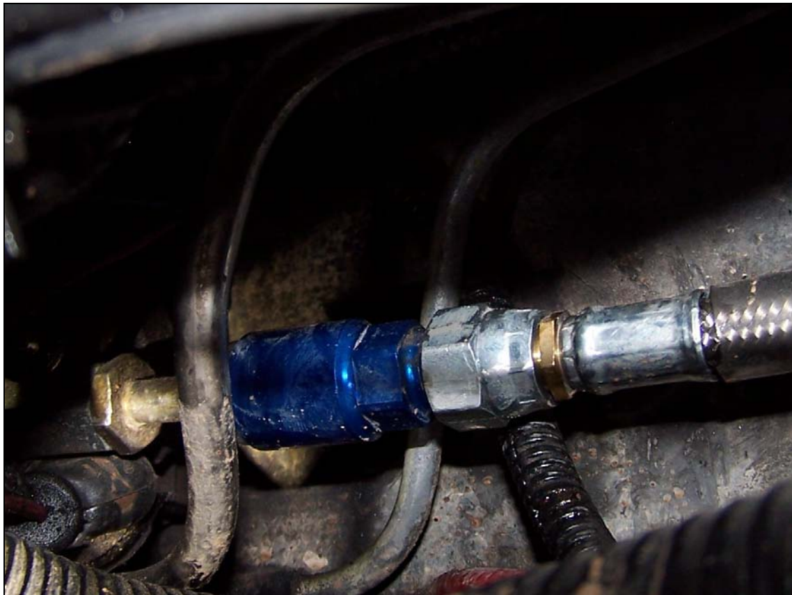
Image 5 – Outlet Adapter (blue in this photo) Installed and Hose Connected (stock fuel pump)
